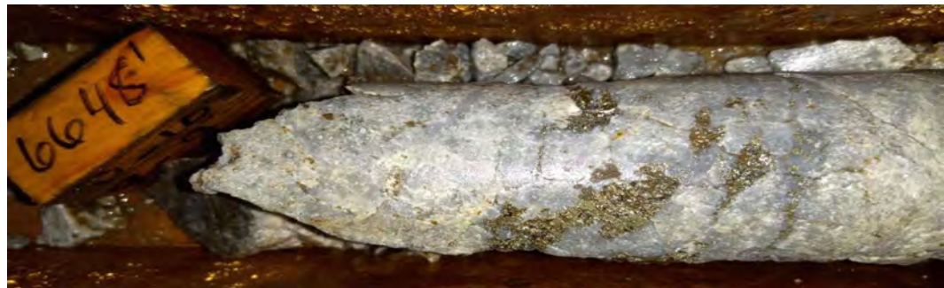
Core from BS-3 at the bottom of the hole (2026.33 m) showing coarse-grained pyrite with quartz, sericite, and minor chalcopyrite (copper-iron sulfide) in quartz monzonite porphyry. High pyrite content, pervasive late-stage sericitic alteration, and high ratios of pyrite to chalcopyrite suggest that BS-3 did not penetrate the copper-rich part of the porphyry system.
