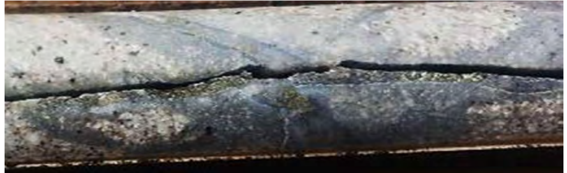
Core from BS-3 (1927.5 m) showing coarse-grained pyrite with quartz, sericite, and minor chalcopyrite (copper-iron sulfide) cutting quartz-molybdenite in quartz monzonite porphyry.
