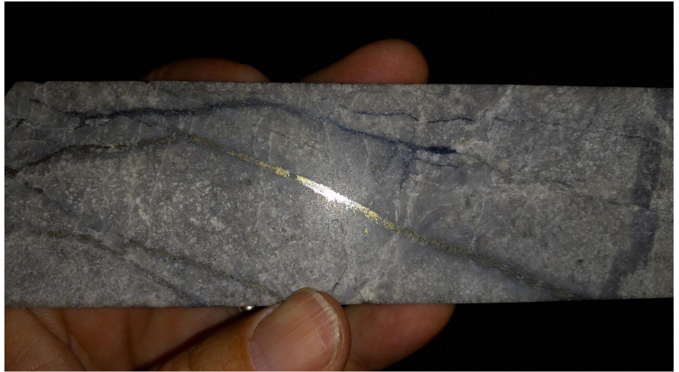
Vein-filling chalcocite (dark gray) and pyrite (brassy) in sericitized porphyry at 1364.5 meters running 2.12 percent copper over 0.6 meters.
