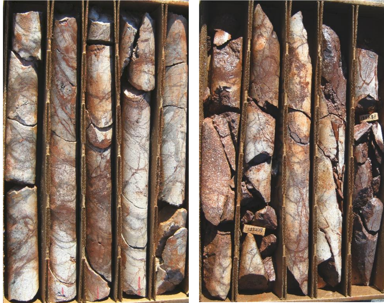
Core box photos representative of the 111 meters of leached capping in BS-3
