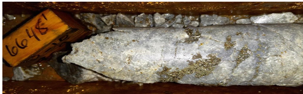
Core from BS-3 at the bottom of the hole (2026.33 m) showing coarse-grained pyrite with quartz, sericite, and minor chalcopyrite (copper-iron sulfide) in quartz monzonite porphyry. High pyrite content, pervasive late-stage sericitic alteration, and high ratios of pyrite to chalcopyrite suggest that BS-3 did not penetrate the copper-rich part of the porphyry system.
