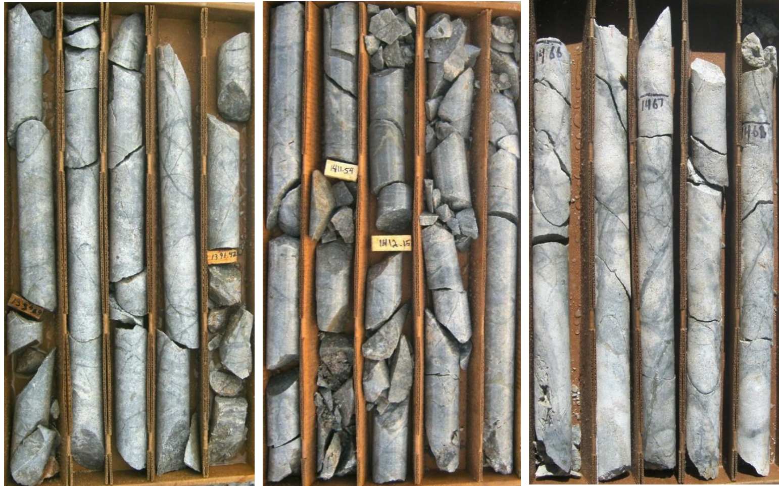
Core box photos representative of the 200 meters of supergene chalcocite mineralization in BS-3
